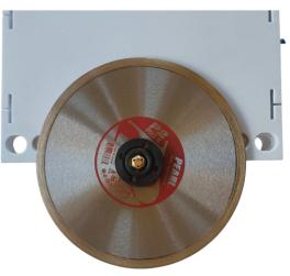
Place saw blade on the threaded arbor. Place blade nut on top of the saw blade.
