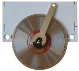
Align wrench with holes on the blade nut and tighten.
